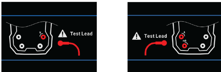
Fig. 9.1 Test lead connection error screens
